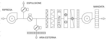
In the adding module can be placed various type of special filters in order to complete the standard filtering section.
